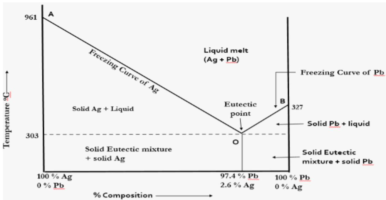
The two metals : Lead and silver are completely miscible in the molten state and they form a homogeneous solution . They do not react with each other to form any compound.
