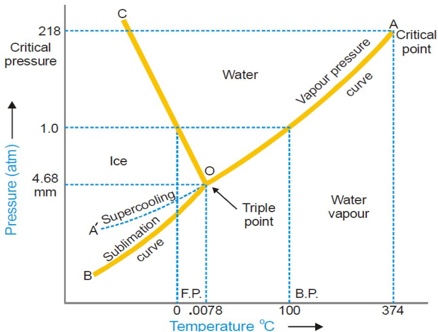
**THE WATER SYSTEM :** This system consists of 3 phases –ice, water, vapour and one component ie  $H_2O$
